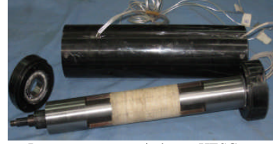
Fig. 6. Permanent magnet-inductor HESG prototype
